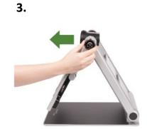
You can switch between modes by rotating/adjusting the camera using the Camera Positioning wheel.
