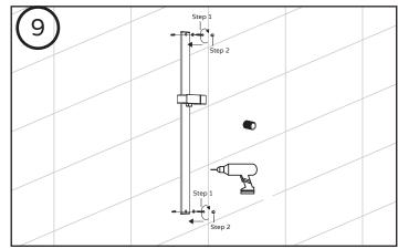
[Step 1] Choose desired position and drill wall anchors into finished wall. Drill in gasket, and mounting screws onto slide bar.
