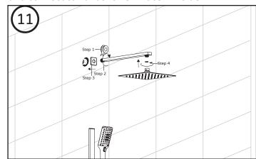
[Step 1] Place plumbers tape on nipple threads.
