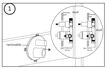
Confirm the installation position and remove the plaster guard.
