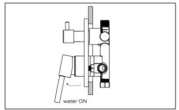
Turning valve ON, lift valve handle up.
