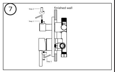
[Step 1] Insert allen wrench into diverter threaded pin and thread to diverter body. Place on top of diverter cartridge, and thread with allen wrench until secure.
