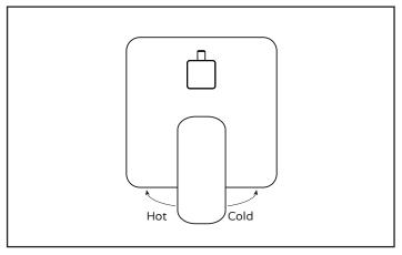
While ON, turn valve handle to the left for HOT and right for COLD.
