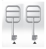
Clamp the rail bracket over the edge of the bed deck with the vertical sliding steel plate positioned on the inside of the bed frame. Tighten the two Allen screws and rotate the turn knob underneath the bracket clockwise until the rail is secured in place. Repeat the procedure to install the bed rail on the other side.
