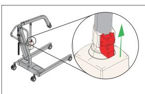
In the event of hand control or control box failure, locate the red handle above the actuator.
