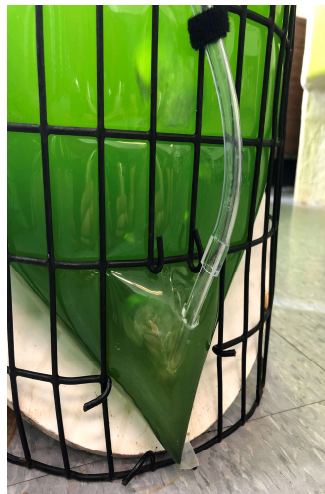
Figure 5: Airline Detail (notice Velcro strap at top)
