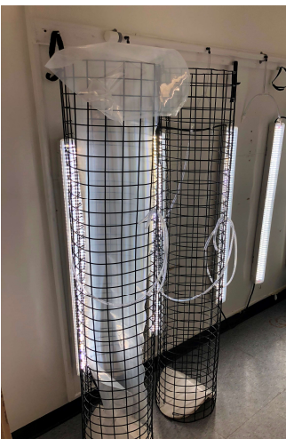
Figure 4: Reactor Cage with LED Light and Plastic Bag
