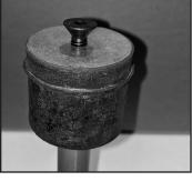
Using the Allen Key remove screw from rubber mount. Fit screw through hole in centre of large 8 inch Flat Disc. Insert the exposed end of the screw back into the rubber mount.
