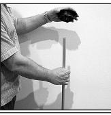
Place the Touch Cap Sphere snugly onto the top of the pole.
