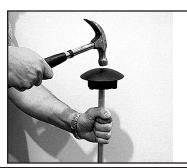
Very Important: Firmly hit the sphere with a hammer or turn upside down and hit firmly against the floor to lock into place.
