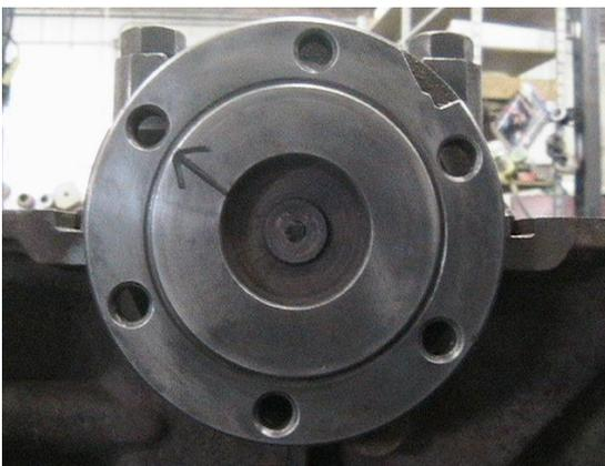
The arrow shows the position of the offset bolt hole.
