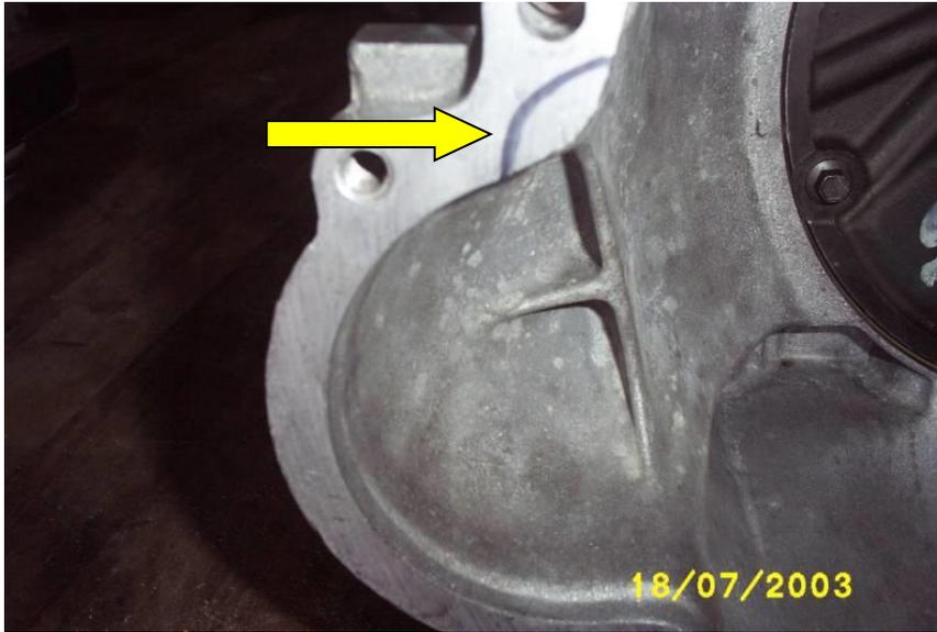
This picture shows where you have to grind the case to clear the starter.
