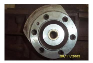
You just need to see this extra hole through the flexplate. It does not have to be perfectly lined up. It is only there for reference.
