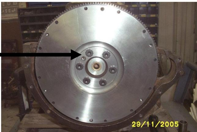
**Make sure you can see the dimple in the crankshaft through the alignment hole**
