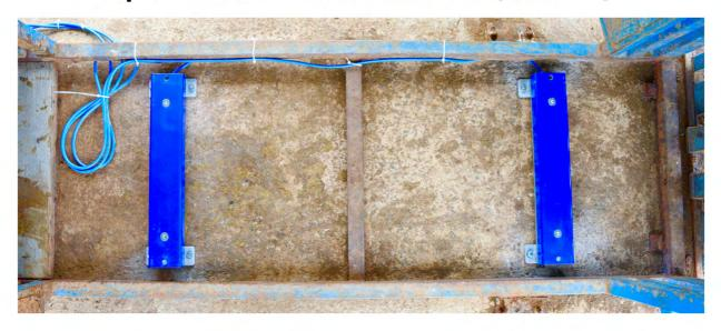
Add 2 x Aluminium Plates (6mm) for Load Bars
