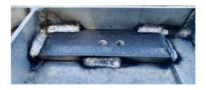
Add the provided spacer and then simply bolt on the 4 load cells with feet and calibrate
