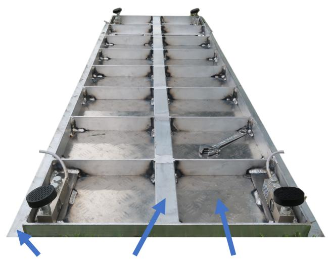
50mm Angle, 50mm Square Tube with 6mm Diamond Tread
