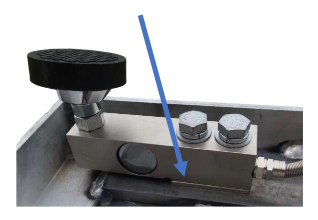
Ensure a good clearance gap is maintained (at least 2mm)
