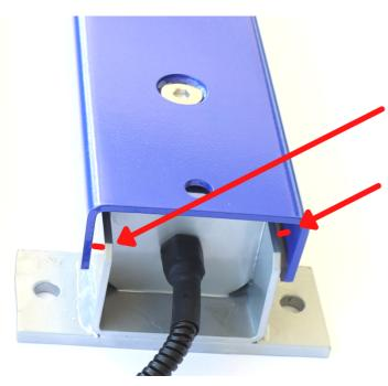
A gap of at least 5mm must be maintained between the floating top section and the main structure for the load bars to work correctly
