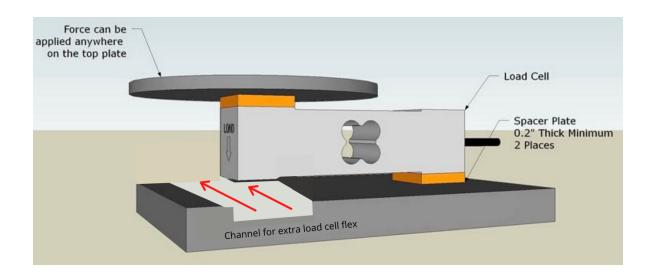
Create a channel for extra load cell flexibility to take accurate readings when installing on a timber platform.
