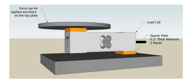
If installing on a timber platform – add a channel so the load cell has more room to take a reading with less chance of touching the platform.
