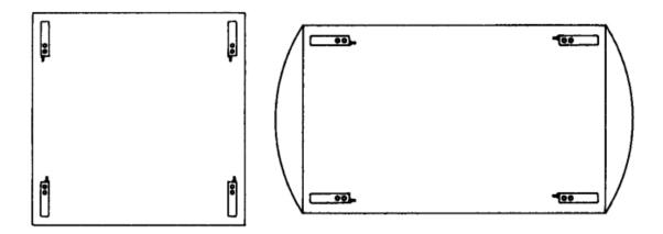
If using steel – weld the (4) mounting brackets provided to the platform prior to attaching the load cells with high tensile bolts.
