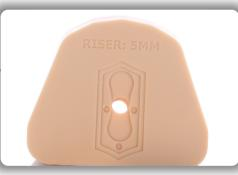
In the case that you have supports on the surface outside of the figure 8 pattern, make sure to clean any excess material from supports to enable flush fitting onto the adapter.
