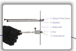
8 Connect the midline bar, horizontal bar, and baseline to the cube. Follow order to correctly assemble the system.
