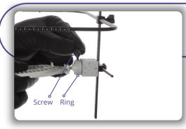
Once everything is aligned, secure the record by turning the ring to the right by pushing the screw. Once the ring is secured, tighten the screw to lock the record.
