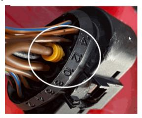
2. Tap newly inserted wire going into PIN 10 of the OEM harness to the yellow wire with blue tracer wire in the same harness using the supplied red tap
