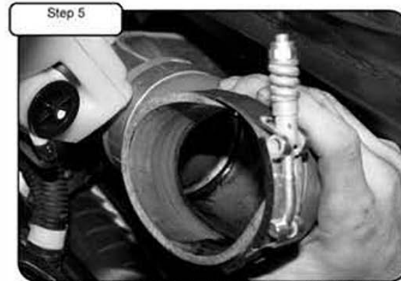
Remove the stock intercooler tube through the fender well.
