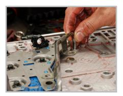
**Step 7**Separate the Valve Body to access
