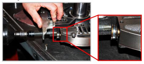
Make sure all valves are free. Remove rotating clutch module from transmission by lifting and wiggle as you lift to avoid disturbing main shaft lube to spacer position. Do not lift up on main shaft. Disassemble rotating module and modify as per Valve body kit instructions. Converter housing on bench provides a nice stand for working on and testing module.
