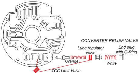
Retainer installs here after TCC limit valve and spring.
