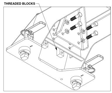
Figure A2: Passenger pivot arm mounting location.
