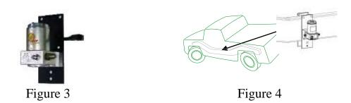
4-3. Assemble the Raptor<sup>™</sup> to the mounting bracket as shown in Fig. 3. Hold the assembly next to the selected location on the frame to check for clearance . Use the spacer block to clear fuel lines or wiring on the frame, adjust the Raptor<sup>™</sup> up or down on the mounting bracket as necessary.
