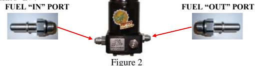
4-2. Install 1/2" O-ring Boss X 3/4" male fitting (08J2044-3/4UNF) into the port marked "OUT". Properly torque the fitting.
