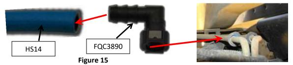
6B-3. Run the fuel line along the frame as mentioned in step 5-3 to the Raptor<sup>™</sup> "In" port. Cut the fuel line to length and insert fuel line end FQC12S per step 5-1. Once the fuel line end is pressed in, connect it to the male J2044 fitting in the Raptor<sup>™</sup> "In" port. A "click" will be heard once properly connected.
