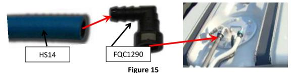
6B-3. Run the fuel line along the frame as mentioned in step 5-3 to the Raptor™ "In" port. Cut the fuel line to length and insert fuel line end FQC12S per step 5-1. Once the fuel line end is pressed in, connect it to the male J2044 fitting in the Raptor™ "In" port. A "click" will be heard once properly connected.
