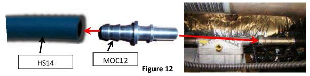
6A-3. Run the other end of the fuel line along the frame as mentioned in step 5-3 to the "Out" port in the Raptor™. Cut the fuel line to length and insert fuel line end FQC12S per step 5-1. Once the connector is installed, connect it to the male J2044 fitting in the "Out" port in the Raptor™. A "click" will be heard once properly connected.
