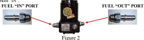
4-2. Install 1/2" O-ring Boss X 3/4" male fitting (08J2044-3/4UNF) into the port marked "OUT". Properly torque the fitting.
