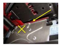
**NOTE:** The fuel tank connections are located behind the tank shield. It may be necessary to remove or bend the tank shield down to access the suction tube quick connect fitting.
