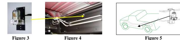
4-3. Assemble the Raptor<sup>TM</sup> to the mounting bracket as shown in Fig. 3. Hold the assembly next to the selected location on the frame to check for clearance (Fig. 4). Use the spacer block to clear fuel lines or wiring on the frame, adjust the Raptor<sup>TM</sup> up or down on the mounting bracket as necessary.
