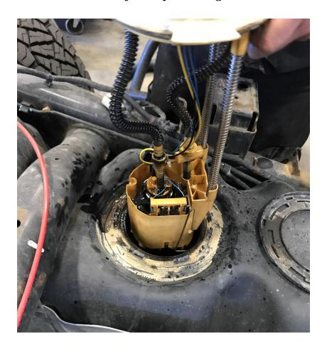
Twist the locking ring counterclockwise to remove and allow for the factory sending unit to slide out.
