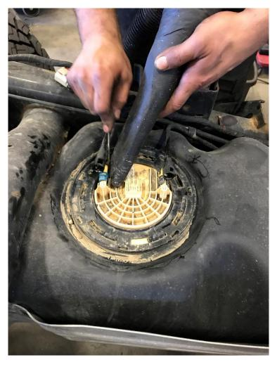
Remove feed and return lines as well as electrical connector
