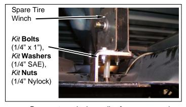
g. Remove two wire loom clips from crossmember.
