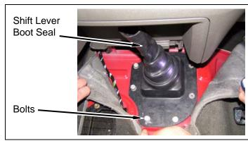
h. Remove two nuts and manual transmission shift lever from shift tower.
