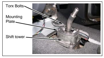
g. Install rubber cover onto shift tower.
