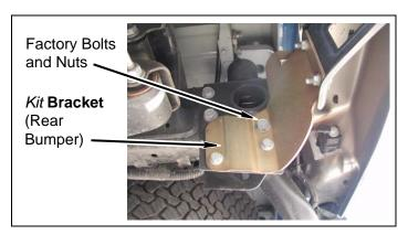
d. Apply small amount of kit Loctite® onto threads of two kit bolts (7/16" x 1-1/2") and install rear bumper onto kit bracket (rear bumper, middle) with two kit bolts (7/16" x 1-1/2"), four kit washers (7/16" USS), and two kit nuts (7/16" Nylock). DO NOT TIGHTEN.
