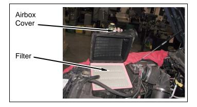
b. Remove nut and airbox from core support and battery box.
