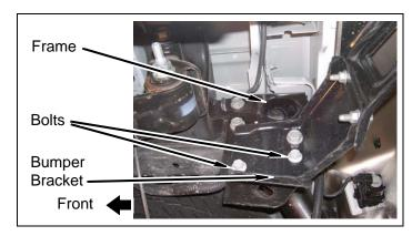
e. Remove two bolts, two captive nuts, and rear bumper.
