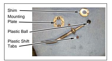
Install shift lever onto shift tower with four Torx bolts.
