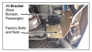
c. Apply small amount of kit Loctite® onto threads of factory bolts. Install two kit brackets (rear bumper) onto frame with two factory bolts and nuts with captive washers. DO NOT TIGHTEN.
