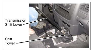
f. Remove six bolts and shift lever boot seal from floor.
