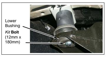
f. **2006 Models:** Install *kit* **bolt** (12mm x 180mm) into each cab mount. DO NOT TIGHTEN.
