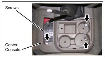
Install transfer case shift lever boot onto center console.
