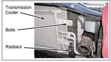
b. Carefully lift transmission cooler from radiator locking tabs.
