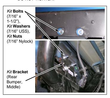
e. Install *kit* **brackets** (rear bumper) onto bumper with two factory bolts and u-nuts. DO NOT TIGHTEN.
