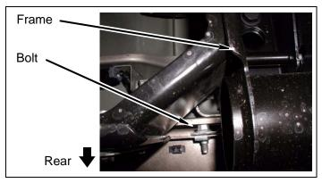
d. Remove four bolts from bumper and frame.
