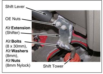
b. Install manual transmission shift lever onto *kit* **extension** (shifter) with two OE nuts.
