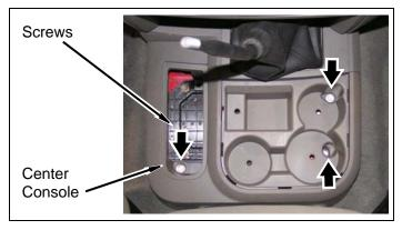
e. Remove manual transmission shift lever boot from shifter console.
