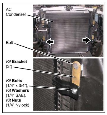
d. Install two *kit* brackets (3" step w/ stud), two *kit* brackets (3"), and AC condenser onto intercooler with four bolts. DO NOT TIGHTEN.
