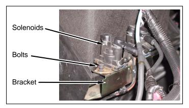
Remove three screws, wiring harness, push clip, and bracket from underneath passenger side battery box.
