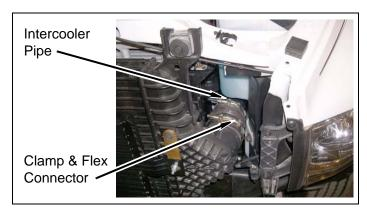
d. Loosen passenger side intercooler pipe clamp at turbo compressor.
