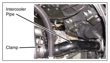
e. Rotate and install passenger side intercooler pipe onto passenger side of intercooler with flex connector and clamp. TIGHTEN two clamps.
