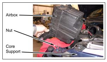
c. Remove two push clip standoffs and AC line from passenger side core support.
