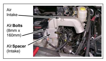
Remove caps and install driver side intercooler pipe, with end marked "top" pointed up, and flex connector onto air intake with clamp. DO NOT TIGHTEN.
