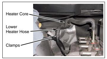
b. Install *kit* **hose** (5/8" x 12" heater) onto heater core and engine heater tube with two clamps.
