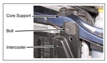
Install flex connector and passenger side intercooler pipe with clamp. Adjust and TIGHTEN two clamps.
