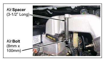
m. TIGHTEN nut and oil dipstick tube onto engine.
