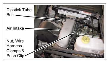
b. Remove four bolts, clamp, and flex connector from air intake and intake manifold.
