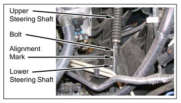
Remove bolt and slide upper steering shaft up to separate from lower steering shaft. Remove brake sensor wire harness from passenger and driver fender wells.
