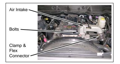
Carefully remove air intake from intake manifold.
