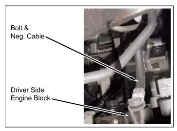
Install kit bracket (angled) onto engine with bolt.
