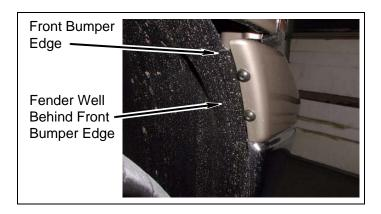
f. Install front bumper onto frame with four kit washers (1/2", thick), two double bolt fasteners and four nuts. Install kit washers (1/2", thick) on bottom bolt of double bolt fasteners, between kit bracket (front bumper) and frame. Snug hardware, but DO NOT TIGHTEN.
