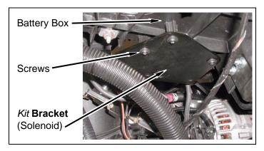
n. Install two solenoids onto *kit* **bracket** (solenoid) with four *kit* **bolts** (1/4" x 1"), eight *kit* **washers** (1/4" SAE), and four *kit* **nuts** (1/4" Nylock).
