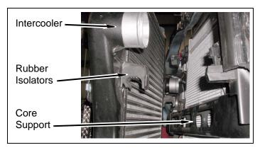
b. Install intercooler onto upper core support with two bolts.
