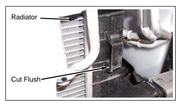
c. Install *kit* **bracket** (cooler, driver) and *kit* **bracket** (cooler, passenger) onto radiator with two bolts.
