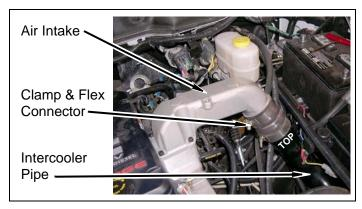
j. Install *kit* **bracket** (3" w/ stud) onto air intake with nut.
