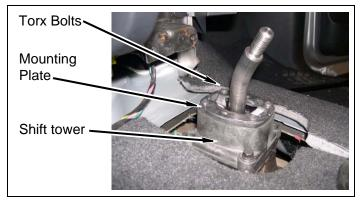
g. Install rubber cover onto shift tower.
