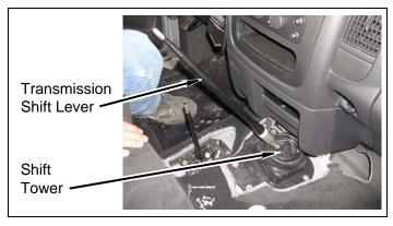
Remove six bolts and shift lever boot seal from floor.
