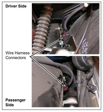
6. Remove two push clips and block heater cord from passenger side frame, if equipped.
