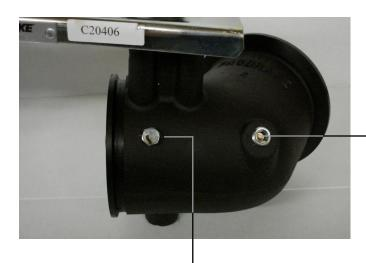
Pyrometer Thermocouple Port 1/4" NPT
