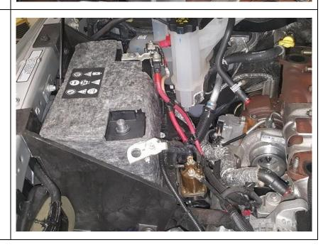
18. Remove the CAC pipe from turbo outlet.
