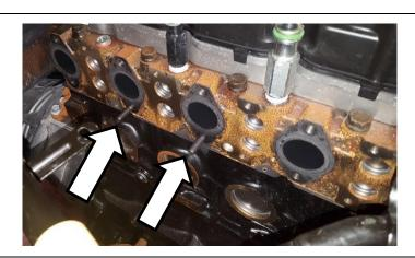
3. Install the 2 coolant plugs. One on the block. Second on the EGR Coolant line.
