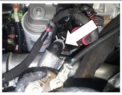
10. Remove the upper turbo coolant line from turbo and engine.
