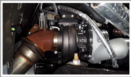
11.Connect the oil feed to turbo (pre-lube turbo prior to connecting feed line).
