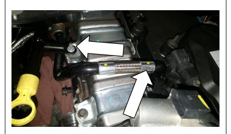
15. Remove the EGR valve assembly by removing the two bolts on side of EGR cooler, two on top and two nuts on the manifold flange.
