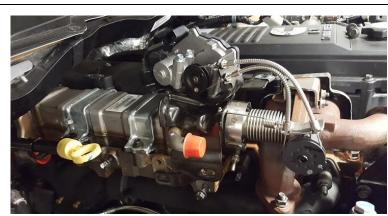
16.Reinstall Coolant stand tube, EGR coolant lines, CCV and EBP sensor.
