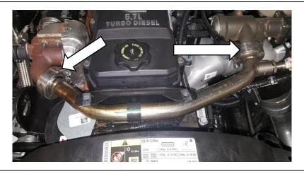
6. Disconnect the two sensors. Note: 2013+ Truck shown.
