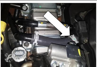
8. Disconnect the two coolant lines at the coolant stand pipe.
