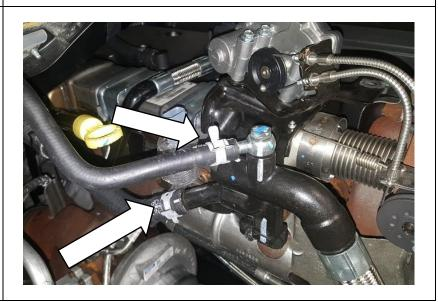
9. Remove the bottom degas bottle hose from bottom of coolant stand tube.
