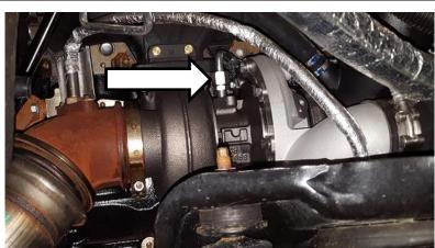
12. Connect the CAC to the turbo. Tighten clamp.
