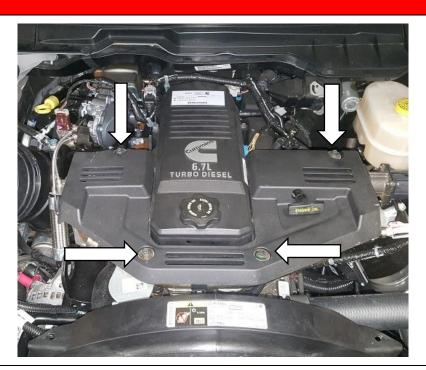
Disconnect sensors and remove the air box and intake hose.
