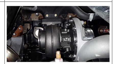
6. Oil drain installation: Drill the mounting holes out with a 25/64" drill bit. Remove the Orings and save. Straighten the major bends a few degrees to lengthen the tube and test fit. Continue to test fit until the bottom seats in the block and top sits correctly on the turbo outlet. Once tube is shaped, reinstall O-ring and install the drain tube with supplied 3/8" bolts and gasket.
