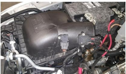
5. Remove the EGR cross over tube by removing the two clamps.
