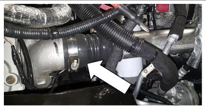
19. Remove downpipe and exhaust outlet casting.
