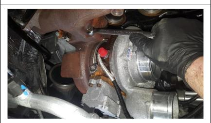
24. Remove the heat shield from the exhaust manifold.
