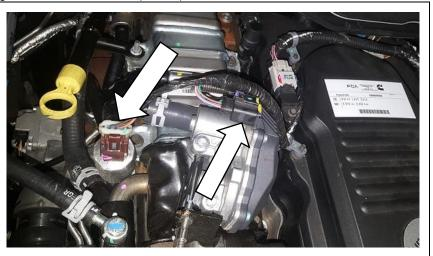
7. Disconnect the hose clamp and remove PCV hose assembly.
