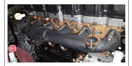
5. Install the turbo onto the manifold. Use the supplied gaskets and nuts.
