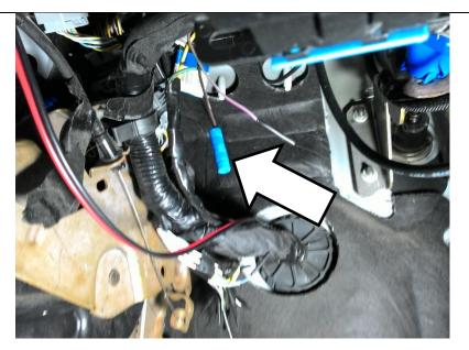
Connect the other side of the posi-lock connector to the RED wire from the BD controller harness. This will supply switched power to the control module.
