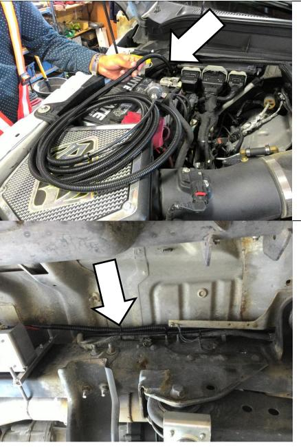
Route it alongside the pump air lines installed earlier and zip tie in place.
