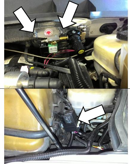
Position the regulator assembly (1220146) over the two M6 studs and install using the supplied M6 washers and nuts. Torque to 50 in-lbs.
