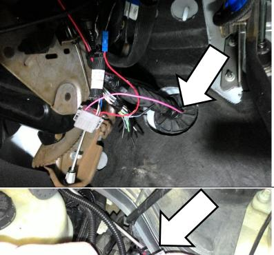
Plug the control module (1304570) into the control harness under the dashboard and secure the module with zip ties below the dashboard.
