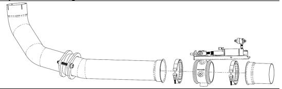
Rotate the exhaust pipes to the correct orientation and rotate the brake valve so that there is sufficient clearance from the vehicle frame, body, transmission etc. Once everything is in place, tighten the front exhaust pipe to downpipe connection and the brake valve clamps. Ensure alignment is still satisfactory afterwards.
