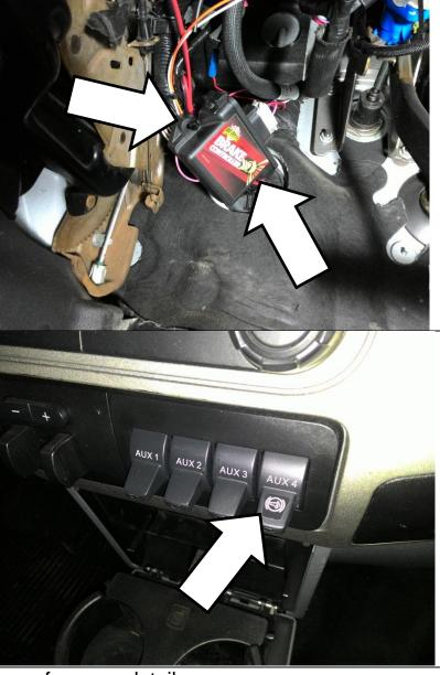
Apply the included exhaust brake decal to the AUX switch used to identify it as the exhaust brake switch.
