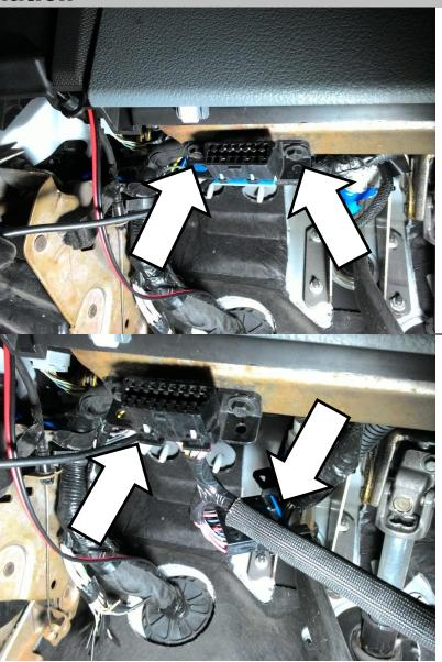
Below the dashboard, locate the up fitter switch wires. These are the four wires located above the e-brake bracket, up by the firewall. Do not mix these up with the larger bundle of wires for the up fitter PTO functions which is below.
