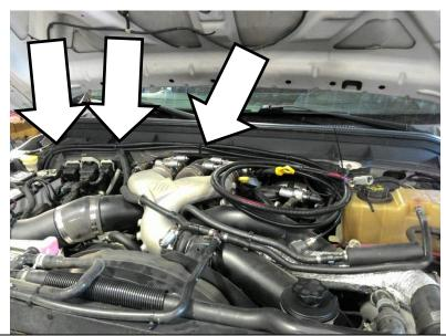
Depending on the routing of the airlines, they may need to be trimmed. The lines are supplied long to account for various line routings. Cut the tubing square and ensure the end is round so it will seal when installed.
