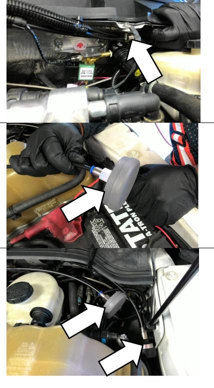
The other line from the air compressor is the suction line, this has the push on fitting to NPT adapter. Thread the supplied "pancake" filter into this fitting hand tight. This is the filter that came with the air compressor.
