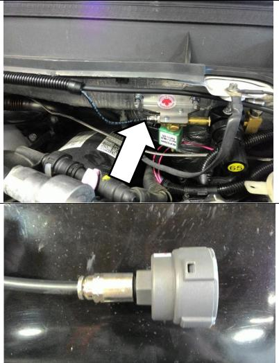
The other 1/4" tube from the brake valve is the vent line. If this is to be trimmed, remove the air filter and reinstall after cutting. Allow it to run past the air regulator assembly, towards the driver side to a dry location under the hood.
