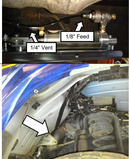
The two sets of air lines and the pump wire will now be left in the engine bay to be hooked up in future steps. Note the lines come up the firewall at the extreme right to avoid the exhaust pipe.
