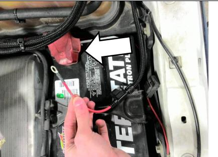
Leave the pink wire from this harness for now, it will be attached to the module output in a later step.
