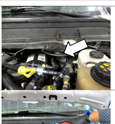
Remove the ground strap bolt on the top of the firewall.
