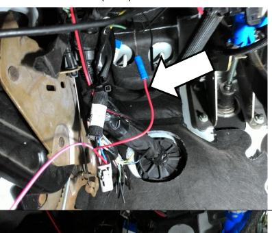
Fish the pink wire from the BD controller harness thru the firewall into the engine bay.
