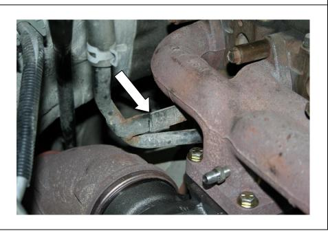
17. Reinstall the *heater pipe bracket* and tack weld back into position.
