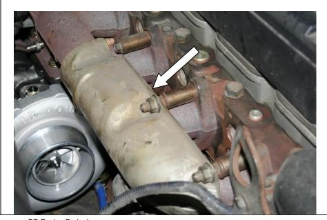
16. Reinstall the manifold heat shield.
