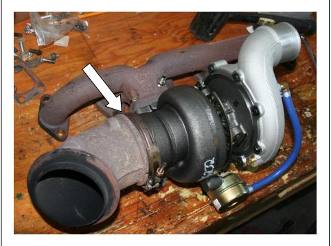
14. Before installing the Killer "B" turbo/manifold assembly clean the surface of the head that the manifold bolts to, and clean out any debris.
