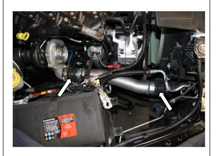
50. Remove coolant fitting from cylinder head with 1" wrench and install supplied pipe plug 3/8" square drive.
