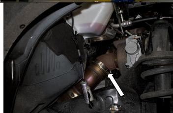
Remove the 2 oil drain bolts (10mm) to extract drain pipe.
