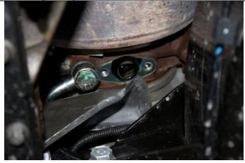
Disconnect intake sensors and remove the intake pipe (8mm socket & pliers) and air box (13mm).
