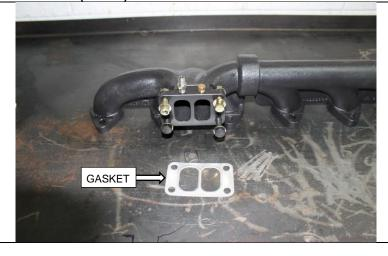
36. Attach turbo to BD manifold using the 2 supplied 3/8" NF X 1.5" bolts, nuts and washers inserted into the drilled holes and (1) M10 x 1.5 x 20mm bolt with flat washer in rear threaded hole. M10x1.5x30mm bolt and washer are used in the front threaded hole. (9/16"or 14mm wrench)
