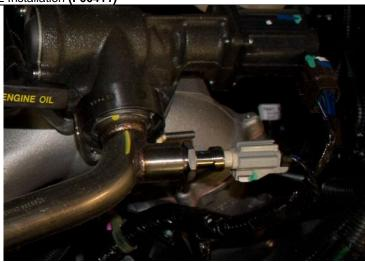
Detach EGR cross over tube, one support bolt (8mm) & two V-band clamps to remove the tube(11mm)
