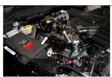
13. Pull out the oil dipstick to remove top engine cover (4 x 8mm bolts). Once cover is removed reinsert the oil dip stick.
