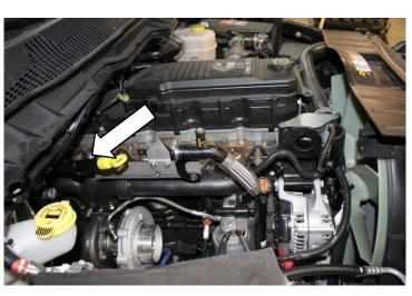
57. Remove and disconnect EGR valve from intake horn.4 (10mm bolts)
