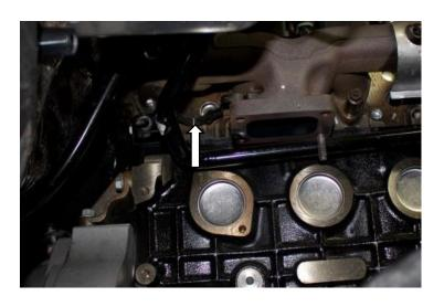
27. Detach exhaust manifold heat shield. Six (15mm) nuts.
