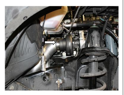
44. Reinstall exhaust hanger onto bell housing.
