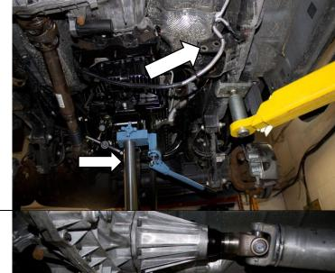
3. Disconnect downpipe at lower joint by transfer case.
