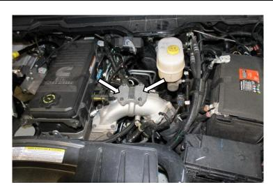
61. Reinstall air box and reconnect sensors. Then install the intake tube with PCV hose and secure PCV to bracket with OEM bolt.(10mm)
