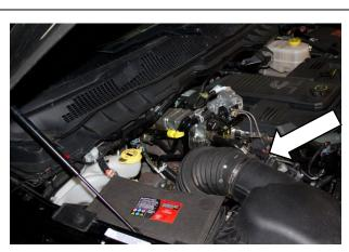
8. Disconnect VGT & speed sensor then remove passenger side CAC pipe.
