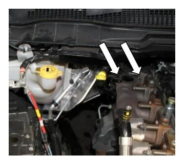
25. Remove 15mm nut and 10mm bolt securing coolant pipe to exhaust manifold.
