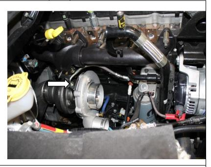
47. Tape VGT Turbo Connections to keep dirt and moisture out.
