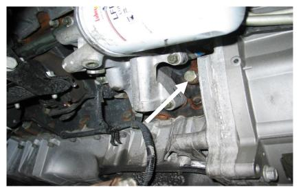
You can now thread the feed line onto the adapter and route the complete auxiliary line up towards the top of the engine. Route the line away from the exhaust manifold, charge pipe and the steering shaft.
