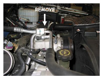
Using a 15mm socket, remove the four A/C compressor mounting bolts to move the A/C compressor for easy access to the turbo assembly. Be careful not to discharge the A/C line.
