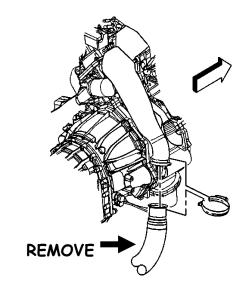
Using a 12mm - **12 point** socket, remove the six upper feed pipe bolts. Note that they may extremely difficult to remove and may require heat to break them loose or penetrating oil.
