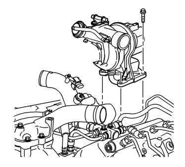
Using a 14mm socket, remove the oil feed line banjo bolt from the center block.
