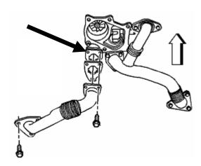
Using a 12mm deep socket, remove the oil drain flange nuts that secure the drain tube to the center of the block.
