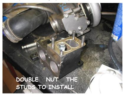
Sandwich the oil drain spacer **1462300** with a gasket on each side (#2405006 and the gasket in the turbo box). Place the oil drain on the bottom. Then Insert the two supplied studs #**1462301** thru the assembly and bolt the assembly to the turbo. Tighten using the 5/16 NF nuts.
