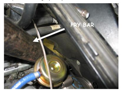
PLEASE NOTE THAT IT IS CRITICAL THAT SUFFICIENT ROOM IS MADE AVAILABLE FOR THE EXHAUST DOWN PIPE. FAILURE TO DO SO WILL CAUSE THE EXHAUST PIPES TO VIBRATE AGAINST THE FIREWALL.
