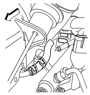
Using a 14mm socket, remove the oil supply line banjo bolt from the top of the turbo.
