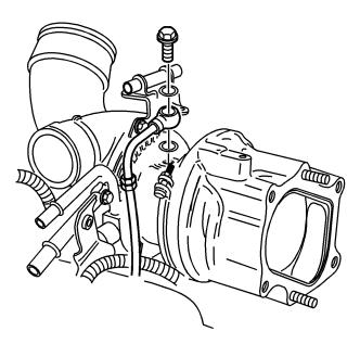
Using a Torx T55, loosen the Banjo bolt holding the lower coolant fitting in place to ease removal. You do not need to remove it.
