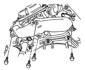
Using a 12mm - **12 point**, remove the four bolts that secure the down pipe to the turbo. As well, you will need to use a 14mm wrench to remove the remaining two nuts from the two studs.
