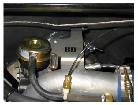
Modify the factory heat shield with a cutoff wheel as shown, stay to the outside of the two spot welds. Install it with two of the three original mounting bolts.
