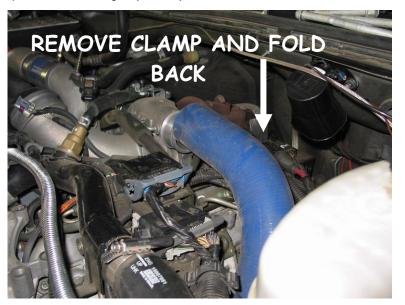
Remove the factory wastegate hose and breather hose using pliers. The breather hose runs from the drivers side valve cover to the passenger side valve cover under the wastegate actuator. Beneath the waste gate actuator you will find a "T" - Disconnect the breather hose at this point and push/pull the line to the side for easier access to the turbo.
