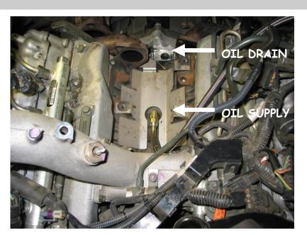
Install the four studs **1462430** into the turbo pedestal by screwing together two nuts onto the studs and tighten the assembly into the pedestal.
