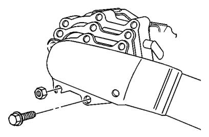
Remove the front curved section of the exhaust from the "4-bolt" flange to v-band clamp. This is located underneath the truck.
