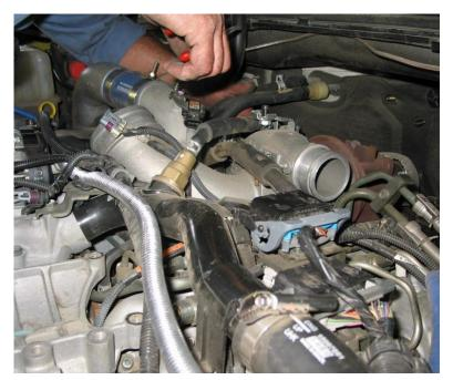
Using a 10mm socket, remove the air intake heater connection, MAP sensor mounting bolt, and unplug the MAP sensor.
