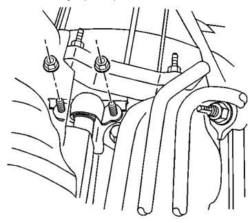
Remove the coolant supply lines from the brass check valve from the top of the engine.
