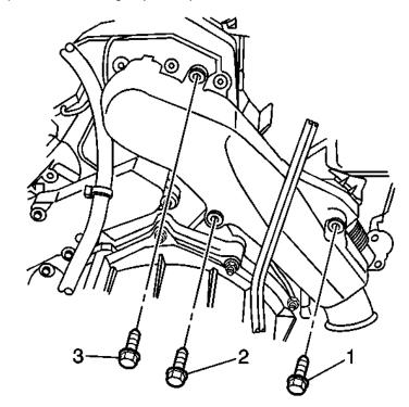
Using a 10mm wrench, remove the four drivers side feed pipe heat shield bolts: three from the top and one from the bottom.
