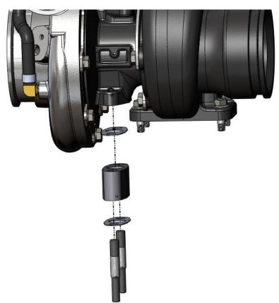
There are three paper oil drain gaskets: two are the same for the upper spacer adapter and one that is different (#1462310) for the tube to engine to block connection.
