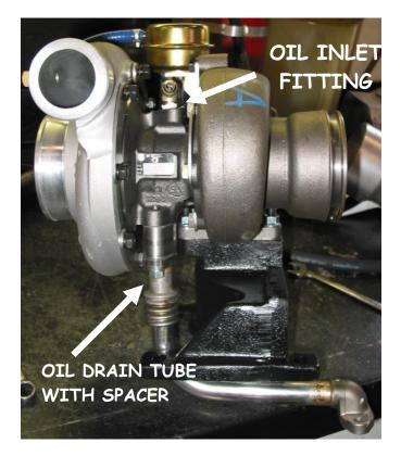
Install the oil drain gasket **1462310** on the two studs on the block. Pay attention to the proper orientation of the gasket. Remove the old gasket residue first before applying the new gasket.
