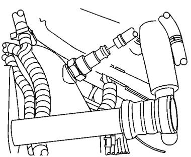
Remove the coolant outlet lines from the turbocharger.
