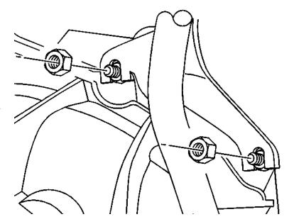
Using a 10mm wrench, remove the three rear heat shield mounting bolts. This will allow you to remove the heat shield protecting the down pipe.
