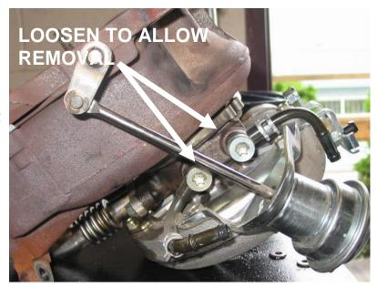
Using an 18mm socket and extension, remove the three turbo assembly mounting bolts. These bolts secure the turbo assembly to the top of the block. Remove the turbo assembly, then the down pipe up through the engine compartment.
