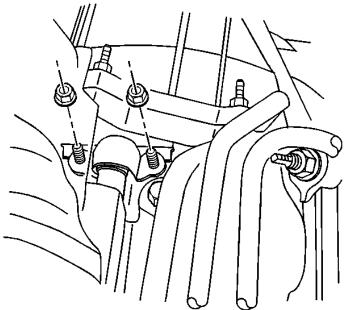
Install the complete turbo assembly (pedestal and all) into the vehicle making sure to align the oil drain flange over the two studs at the rear of the engine. Tighten to **15 lbs-ft** of torque.
