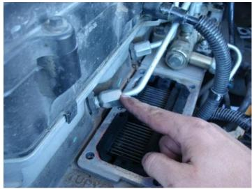
16. Disconnect the Intake air temperature sensor connector from the grid heater.
