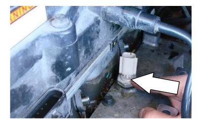
24. Remove the four remaining bolts that hold the grid heater to the engine.
