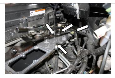
Reconnect the fuel rail connector. Then apply some pipe dope to the four OEM fuel rail bolts and reinstall the fuel rail to the intake plate. Torque to 18 ft/lbs. (10mm socket)
