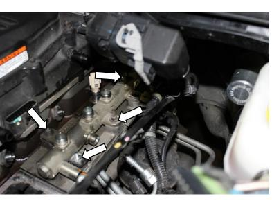
22. Disconnect the Fuel rail connector from the back of the rail, the rail can now be removed from the vehicle.
