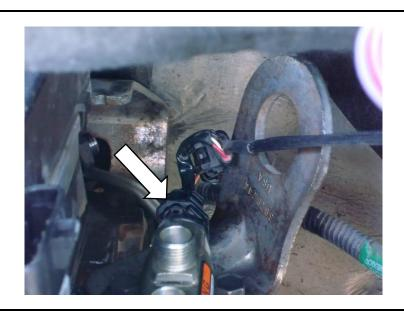
23. Using the 1" wrench remove the IAT sensor from the grid heater.
