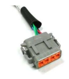
Remove the orange lock wedge from the Throttle Sensitivity wiring harness using needle nose pliers.
