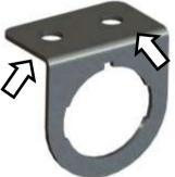
Apply the "Throttle Sensitivity" decal to the dash or button bracket, then install the button. To make button installation easier the tabs on the button can be squeezed down while inserting into the dash or bracket using a small screw driver or pick.
