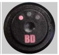
To activate valet mode, press and hold the button for five seconds. All three LEDs will light up. The module will now limit vehicle power until it is taken back out of valet mode. To turn valet mode off, press and hold for another 5 seconds.
