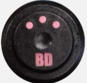
To activate "ludicrous speed" mode, press and hold the button for 10 seconds until all of the LEDs begin flashing. To leave this mode, simply press the button once. This mode will turn off by default on the next start for safety.
