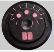
The module will automatically detect if the button is attached. If the external button is disconnected from the module, it will default to the mode selected on the switch inside the module. The button can be connected or disconnected at any time after the module is installed. If the external switch is connected it will override the internal module switch.
