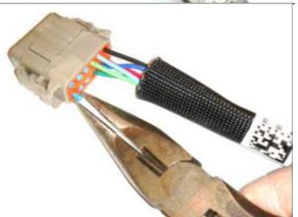
Insert the wires from the BD Button wiring harness supplied in this kit into the gray connector according to the chart below.
