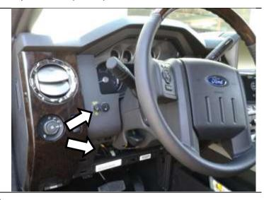
If installing in the dashboard, ensure there is space behind the chosen location for the button depth and the wiring connector to be attached. Ensure nothing is behind the chosen location that may be damaged while drilling the dashboard. Create the mounting button hole using appropriate sized drill bit or a stepped drill bit. Then using a small file, create a notch at the top of the hole for the button locating tab to go. Use the button bracket for reference.
