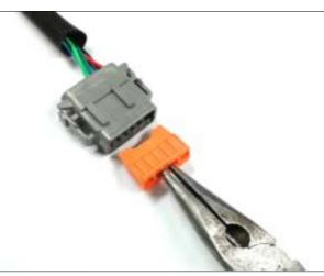
Remove the small plastic plugs from the back of the connector using needle nose plyers or a small pick and discard them.
