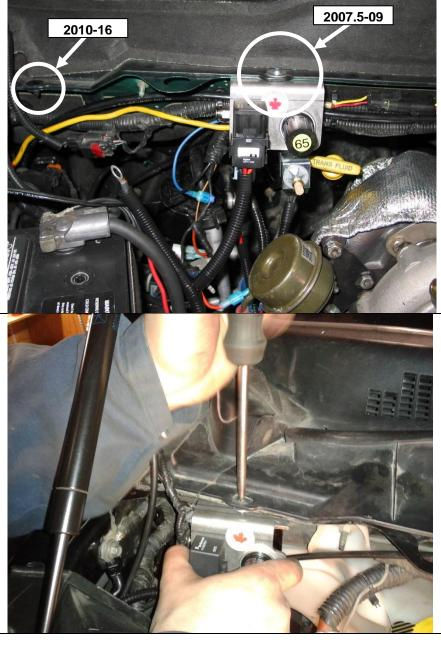
2010-2019 Vehicles Remove the plastic trim clip or wiring harness clip on the top of the firewall near the coolant bottle. This hole will be used to install the regulator assembly.
