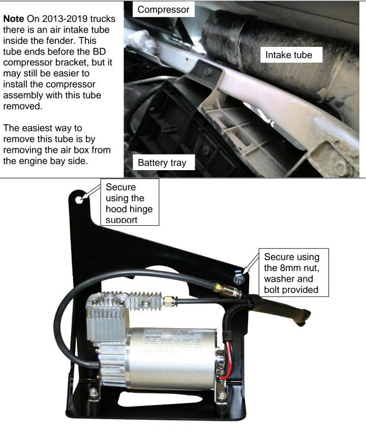
Feed the compressor air lines and wire through the fender into the engine bay, they will be connected later. Lift the compressor into place.
