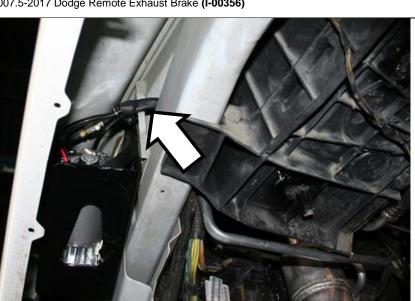
Secure the compressor in place by reinstalling the hood hinge bolt through the compressor bracket. Then install the nut and bolt to hold the front of the bracket.
