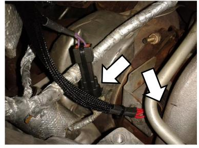
26. Reinstall the intake manifold. The old gasket may be reused if it has not been damaged.
