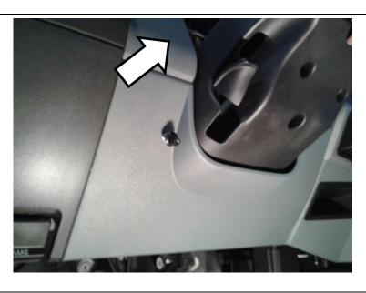
12. Drill a 7/8" hole in the dashboard with a stepper bit or hole-saw. Using a small file, create a notch for the locator tab of the switch. Clean up the edges of the hole as necessary with the file.
