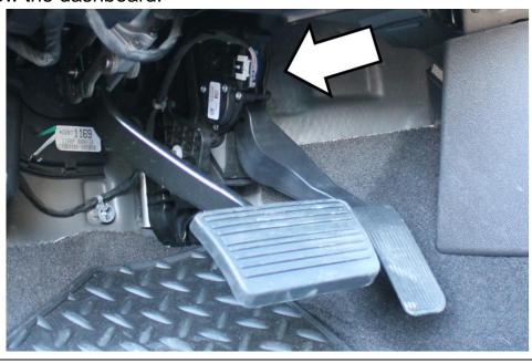
3. Connect supplied wiring harness to the accelerator pedal position sensor and the other end to the factory wiring harness. Secure harness with zip ties so that it does not interfere with pedal operation. Removal of the knee bolster may ease installation.
