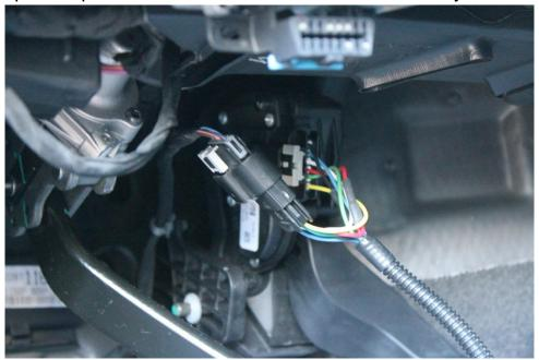
4. For 98.5-04 Dodge kits, disconnect the control knob harness from the main wiring harness. Route the small disconnect wire through the firewall and reconnect it to the main wiring harness. (Not required on other models).
