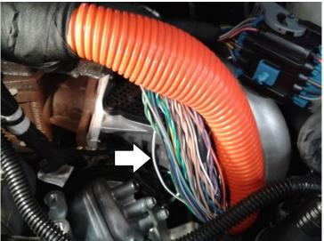
**2017-2018 GM L5P** – Locate the 8 pin sub-harness disconnect on the top of the engine for the crankshaft position sensor. Locate the solid green wire in pin 3. Remove some harness tape to have some wire to work with. Attach the light blue wire here for RPM pickup. Solder the wire and cover with heat shrink for longevity. Rewrap with tape when complete.
