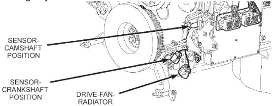
**2014-2018 Dodge 3.0L (EcoDiesel)** - Locate the engine crankshaft position sensor connector. This is located in the rear of the engine oil pan, just ahead of the transmission as shown in the picture. Tap the brown wire with light blue tracer (connector pin 3). Solder this connection and cover with heat shrink for longevity.
