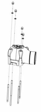
Insert the 4 M6 Acorn nuts onto the studs and torque to 8 ft-lbs (96 in-lbs).
