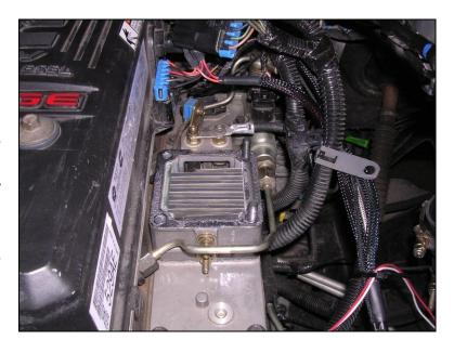
With the jam nut supplied you will need to double nut each stud and torque the stud down in place to 3 lbs-ft. You must make sure that the threads are fully seated in place. Once it has been torqued, you can remove the two nuts.
