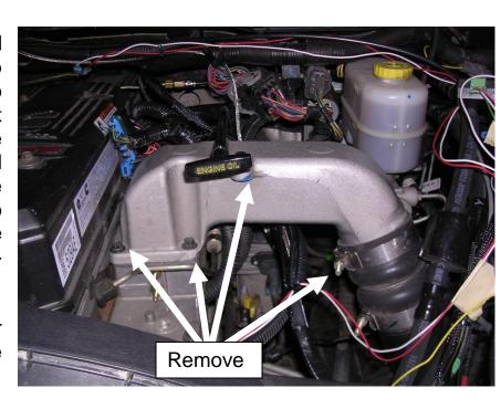
On the rear of the intake you will notice a wiring harness bolted to the intake. You will need to remove the nut and washer that secure the wiring harness to the intake.
