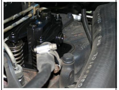
3. Inspect the valve cover bolt and remove the oring that sits underneath the bolt head.
