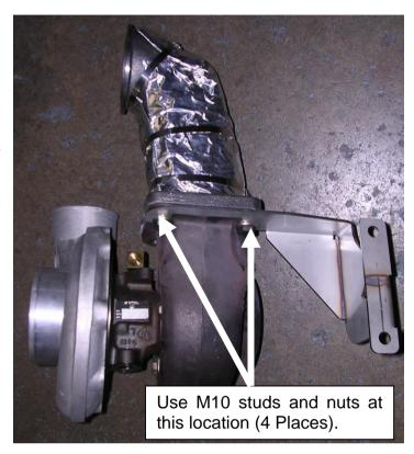
30. Place the turbo and turbine adapter assembly onto the frame rail in a location close to the final install point. Be sure that it does not fall.
