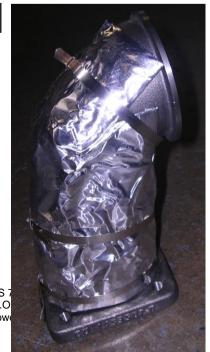
shield has been formed in a specific pattern to completely wrap around the elbow. Use the 3 supplied stainless steel zip ties to secure the heat shield. One at the bottom, one at the middle and one at the top. Be sure that neither the heat shield or zip tie will interfere with the circular marmon flange when the band clamp is applied.
