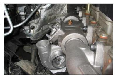
31. With the secondary turbo, bolt it loosely to the manifold and align the oil inlet straight up and the compressor outlet towards the bottom of the passenger battery.
