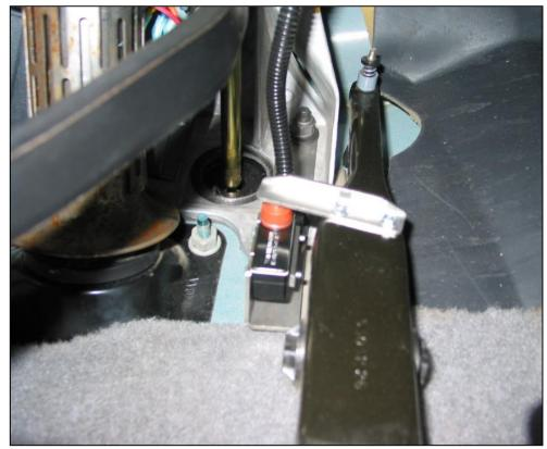
The arm of the throttle pedal starts off wide, then angles off into a thinner section further up the pedal.
