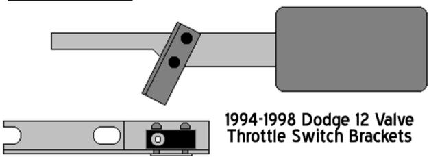
At the throttle pedal, locate the nuts on the large aluminum bracket, just up from and to the left of the pedal. These nuts secure the aluminum bracket to the firewall and are the mount for the throttle and brake pedal. Remove the lower nut and loosen off the top nut. In the kit you will find the long throttle switch bracket, which has two long slots for the throttle switch.
