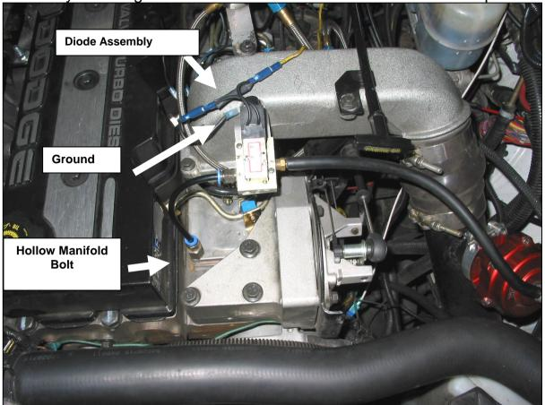
When securing the spool valve assembly with the long 10mm bolt, connect the spool valve ground (ring connector) between the intake horn and the spool valve assembly. Be sure to re-torque the 10mm bolt, or a boost leak may occur. Install the "Free Wheeling" Diode pigtail assembly. Route the power through the red wire and then into the spool valve. The black wire of the assembly should be mounted to ground using the ring connector.
