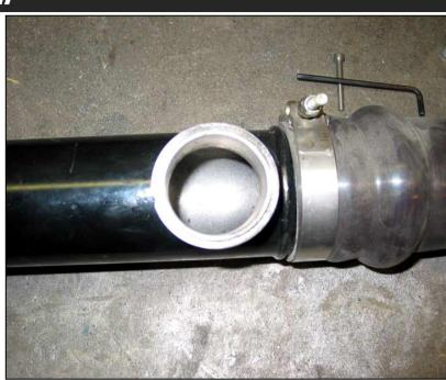
As you can see from the picture above, the edge of the adapter should be within a ½ inch from the second raised lip. Once you have marked your drill location, use a center punch and drill a pilot hole. Use a 1-7/8" hole saw and drill out the remainder of the hole.
