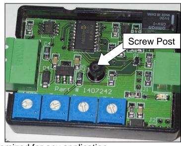
Now adjust the APPS potentiometer to reflect your desired activation point based on the amount of throttle released. Remember if you would like the valve to activate only when a large amount of throttle is release turn the dial clockwise. Conversely turn the dial counter clockwise if you want the valve to activate on smaller amount of throttle release.
