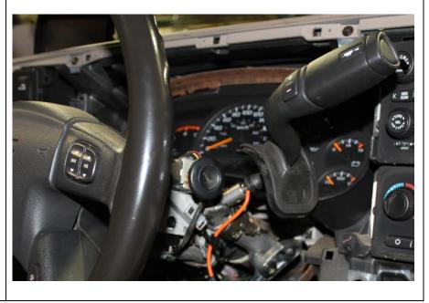
8. Reattach new lever with existing torx screw.
