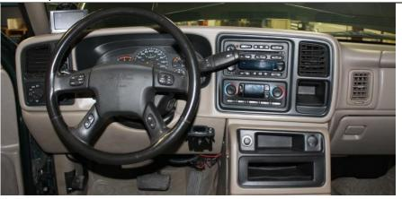
20. Clip the TCM back into its cover and temporarily reinstall it (you can leave the mount screws out). Route the Tap Shifter harness with the BLUE and BLACK connectors to this location. Choose a spot on the TCM cover to mount the Tap Shifter module and mark the locations to be drilled.
