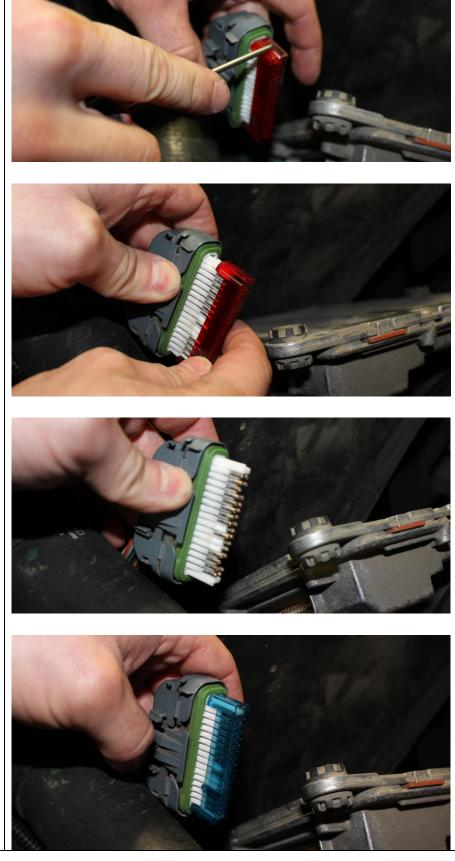
11. Remove the RED retainer on the vehicles transmission harness connector. Install the supplied BLUE retainer. Keep the removed RED key incase the module is ever removed. 12. Connect the BD Tap Shifter wiring harness RED connector to the vehicles transmission control module.
