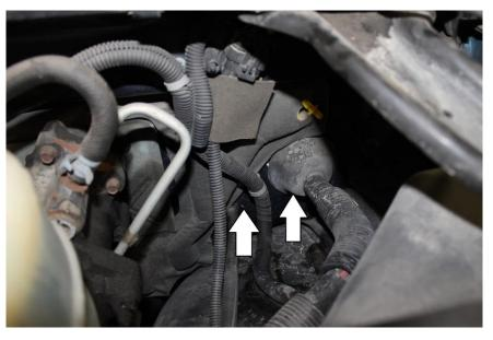
15. Connect the new wiring harness to the shift lever and to the vehicles original shift lever connector. Depending on harness routing in the engine bay, there may be excess wire. Coil wire out of the way of the pedals if necessary.
