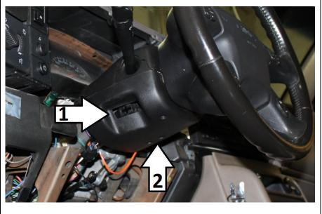
6. Disconnect the two pin electrical connector running to the original shift lever under the steering column. Remove the two plastic clips holding the shifter wire to the column.
