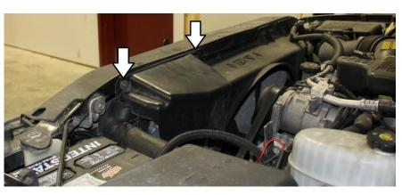
10. Unclip the transmission control module from the cover if required for access. Disconnect the top (RED) electrical connector.
