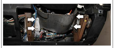
Remove the tilt lever from the steering column (1) and the screws from the bottom side (2). Unclip the upper and lower covers. Use care not to break the clips on the covers.
