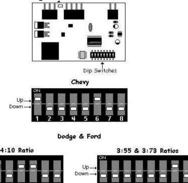
**NOTE:** To insure proper function of the dip switches, flip each dip switch back and forth once before setting them, even if the dip switches are already set for the application it's being installed on.
