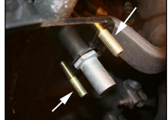
Install the bearing assembly over the sector shaft nut until the bearing block comes to rest on the support bracket (noting that the block may not be flat to the mount at this point).
