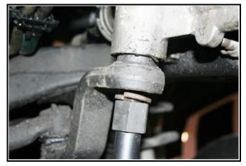
Slide the support bar into place, where the mounting feet are positioned in between the sway bar mounting and the frame.
