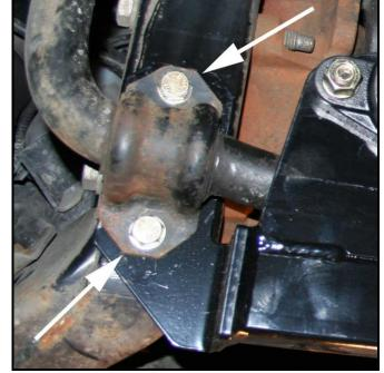
Remove the set screws and apply LocTite.
