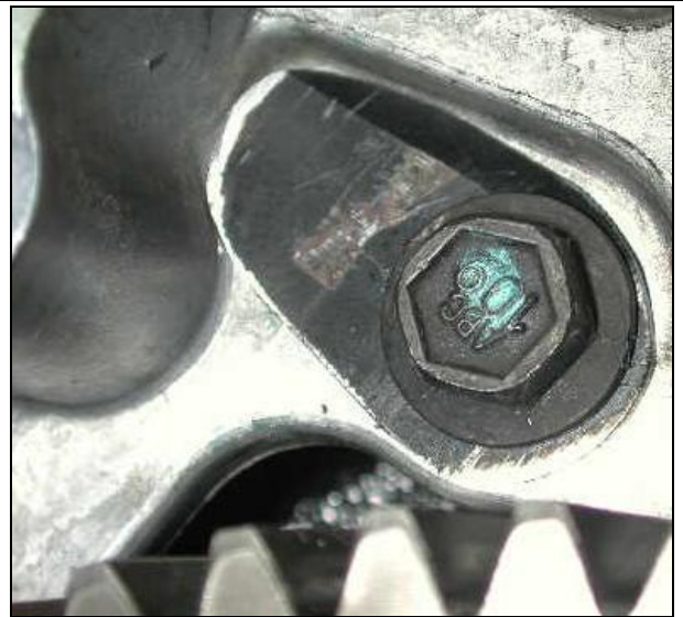
With retainer and bolt installed
