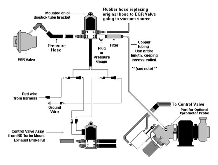
\*\*NOTE\*\*: Ensure that the copper tubing is properly secured to prevent breakage.
