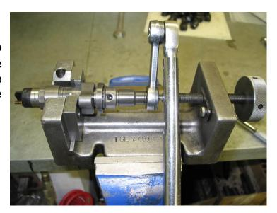
Slide down lock ring to the lower land and insert new O-Ring. Also install new copper washers on the base of the injectors.
