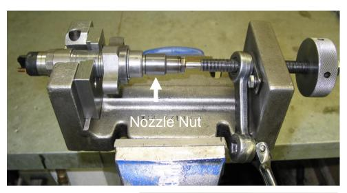
Once the nozzle nut is removed, clean any debris/carbon soot build up on the inside of the cap. Also check the injector body for any cracks or unusual wear.
