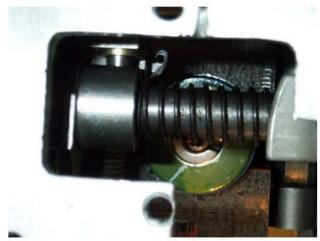
17. Using Vernier calipers, measure the distance from the top of the governor stud to the top of the governor spring adjusting nut. Record this measurement for reassembly.
