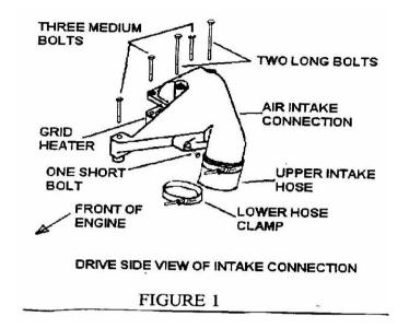
6. Remove the six bolts holding the air intake connection and dipstick tube in place using a 10 mm 6 point socket.
