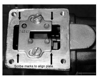
16. Bar (roll) the engine over until the governor spring adjusting nut is just to the left of (below) the rocker strap.
