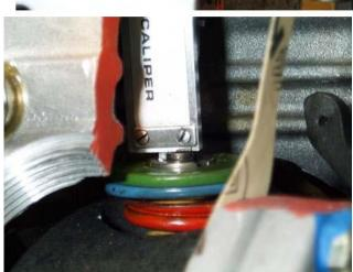
18. Remove adjusting nut using a long thin screwdriver and a pencil magnet.
