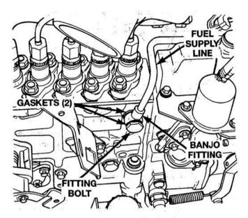
Fuel Inlet Line at Injection Pump
