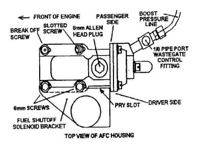
11. Mark the position of the AFC housing on the pump then, using a hand impact tool and an 8mm socket, remove the two driver side AFC screws. Then loosen 8mm bolt on the governor cover to free the shut off solenoid.
