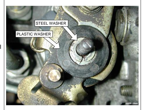
20. Clean and grease the throttle lever bolt and reinstall the throttle lever, throttle rod, and return spring. Reinstall the APPS sensor and linkage if so equipped. Start the vehicle, check for fuel leaks and road test.
