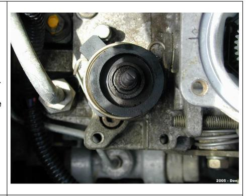
4. Remove the tamper-proof cap on the high idle screw. Simply grab it with pliers (it will crush when you do this) and pull towards the rear of the vehicle. You may need to give the pliers a tap with a small hammer.
