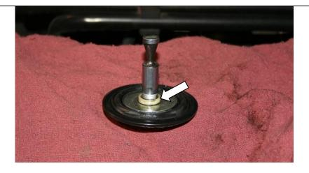
7. Carefully note which way is "up" on the rubber diaphragm (the ridge on the diaphragm faces down). Remove the factory fuel pin from the diaphragm using two 10mm wrenches (or a wrench and a socket). There is a pair of flat spots near the top of the fuel pin that accommodate a wrench. Again, be careful not to damage the diaphragm.
