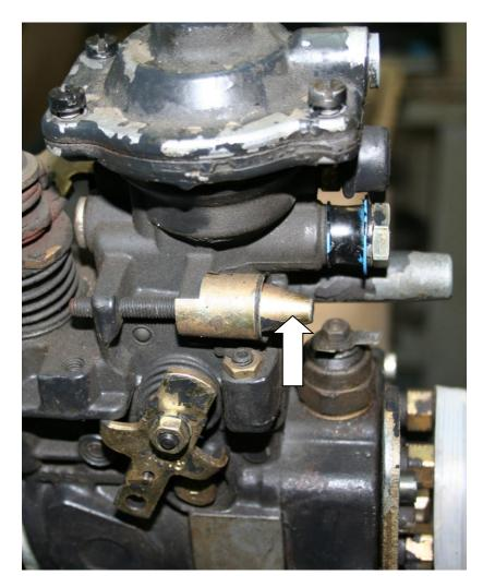
5. Using a 10mm socket, remove the jam nut that secures the remainder of the tamper proof cap. Throw away the tamper proof cap pieces.
