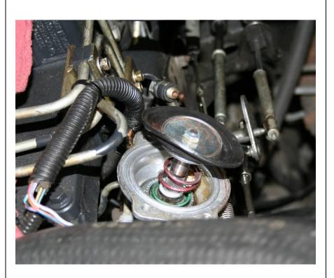
11. To ensure that the machined notch is correctly positioned lift the fuel pin slightly and bring the throttle linkage to full throttle while gently turning the fuel pin & diaphragm back & forth slightly. You should feel a spot of no resistance through the center point of the turn as the guide pin comes out of contact with the fuel pin: this center point is the desired fuel pin position.
