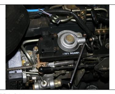
Remove the last slotted screw securing the AFC cover to the pump, remove cover.
