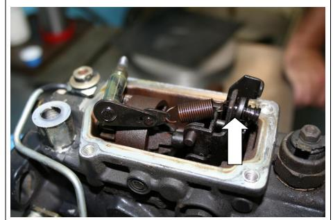
**12.** With the cover off you can now see the governor spring. Carefully inspect its linkage for any cracks or broken pieces; any repairs will need to be done by a professional. Unhook the throttle shaft from the governor spring and replace the throttle shaft o-ring with the one supplied in the kit. A small pick is handy for this, but be careful not to damage the new o-ring (#1505020).
