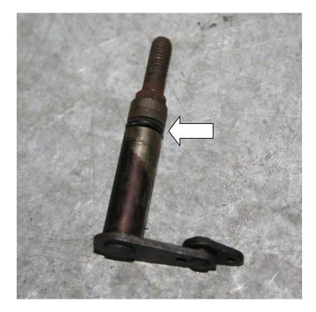
**13.** To change the governor spring simply unhook it from the small springloaded stud inside the pump and hook the BD spring in place.
