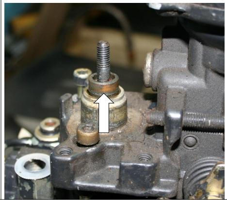
**15.** Now reinstall the main fuel screw back into its previous position, then reinstall the fuel return and AFC banjo bolts.
