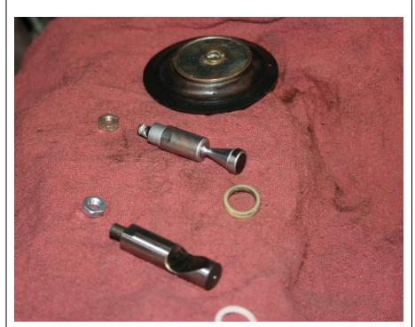
9. Before reinstalling the fuel pin and diaphragm inspect the AFC chamber and make sure the guide pin is clean & will retract all the way into the housing. You may need to stroke the throttle linkage back and forth slightly. Lubricate the guide pin with some diesel fuel.
