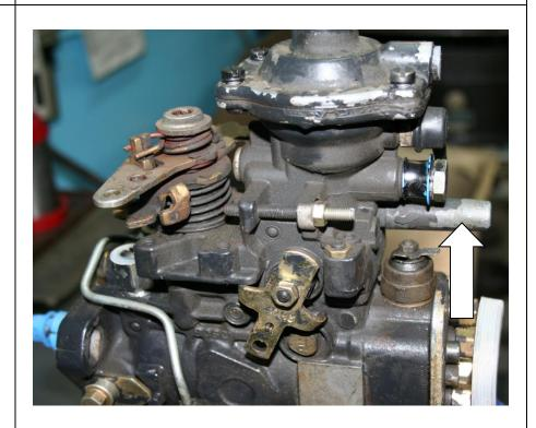
7. Use a 13mm deep socket to loosen the check nut on the main fuel screw then use a 6mm socket or small flat blade screwdriver to turn the screw out until the o-ring is visible.
