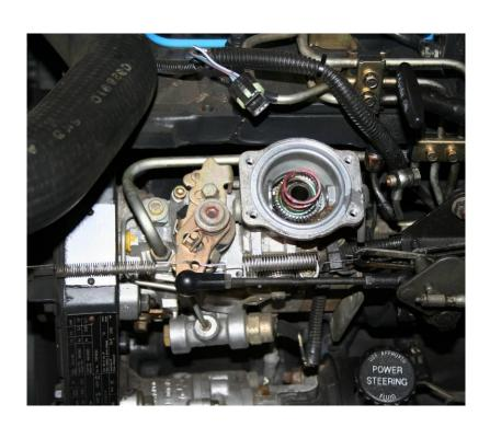
10. Place the supplied black nylon bushing onto the fuel pin so that it is up against the underside of the diaphragm. Lubricate the fuel pin with a small amount of clean diesel fuel and install it into the pump with the machined notch facing towards the front of the vehicle (the guide pin rides on this surface).
