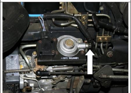
**3.** Remove the (3) APPS sensor / AFC Cover bolts and bracket.
